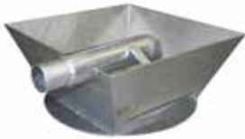
Galvanised Tank Funnel with 455mm Rim. 2" Air Gapped Fill Point and Mesh Grate.
